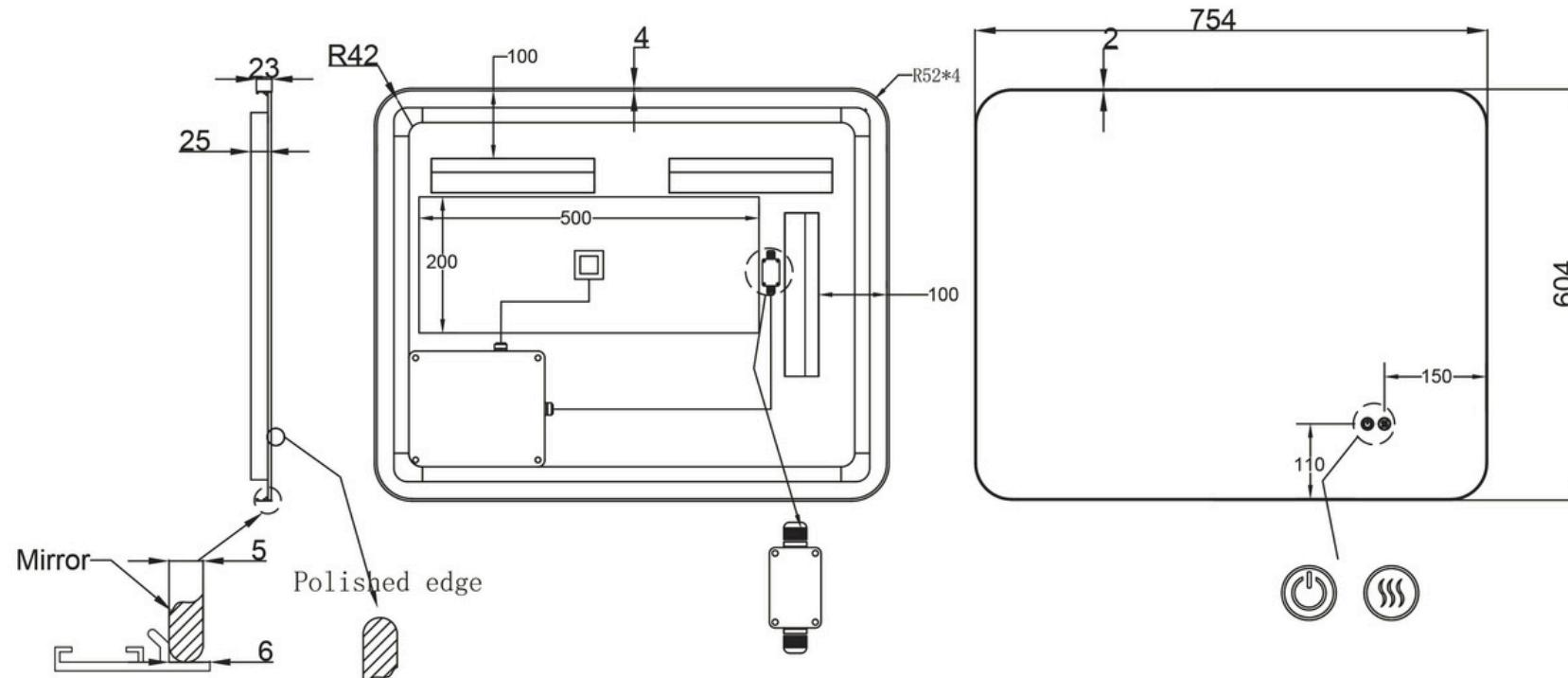
All measurements are in mm and are for reference only. We recommend using a physical product for final measurement and rough-in stages. While we aim to have all measurements perfect at the time of publication and production normal manufacturing tolerances are to be expected and technical drawings may differ from actual product.
